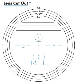
\*PLEASE NOTE: The fitting cross for SOLAOne progressives is 4 mm above the prism reference point.
